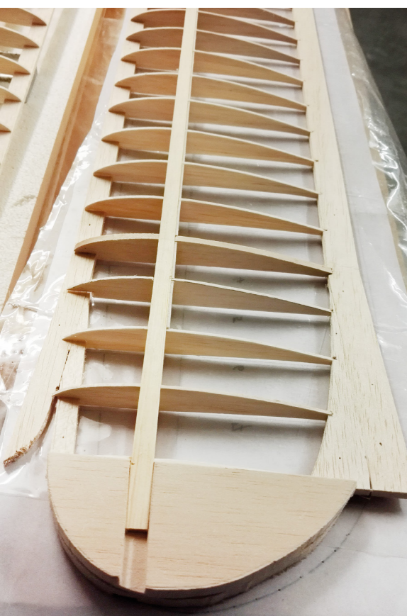
The end strip on the wing ear is still laminated - or you assemble it from individual pieces.
