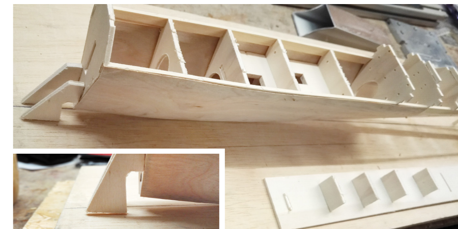
Use auxiliary supports to hold the hull to the slipway.
