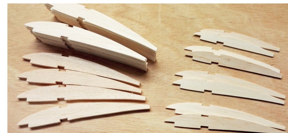
The ribs can be made in a block or - if you want it to go even faster - you can use the milling parts kit available from VTH.
