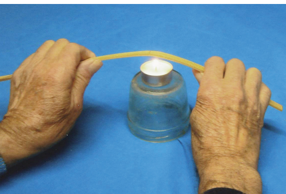
Pre-bend the main spars (pos. 9) over a candle and check the work by laying them on the slipway.
