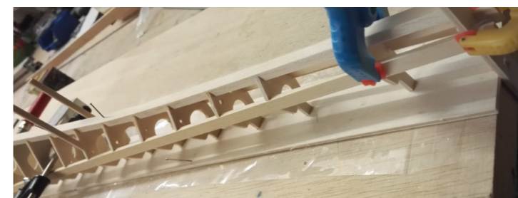
To glue the longitudinal chords, clamp the components with clamping screws and pliers.
